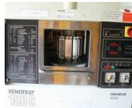
Test chamber for UV test.
