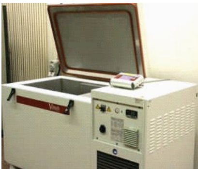
Test chamber (temperature range from -70 °C to +80 °C).
