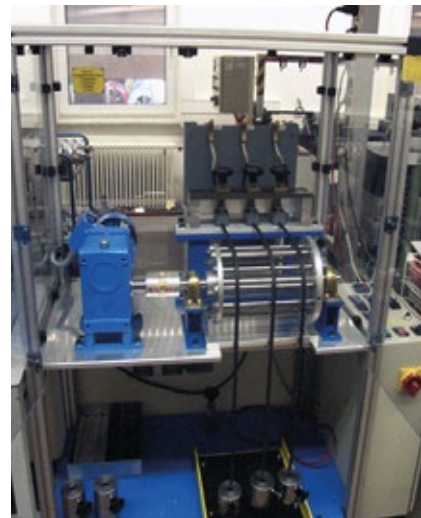
Test cage: Sheath against metal/plastic.
