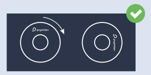
• When only a portion of the cable is used, the open end of the cable remaining on the drum should immediately be re-sealed to prevent the entrance of moisture. Once it has been resealed, the cut end should be fixed to the inside edge of the drum flange to prevent the end from extending beyond the flanges during drum movement.
